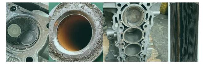
A study conducted by Makassar State University (UNM) in 2019 found that out of 43 diesel cars that experienced damage, 3 had injector issues and 43 had fuel filter damage. Damaged fuel filters were caused by the entry of foreign particles, resulting in dirty and clogged filters from deposits. This caused a decrease in the fuel supply from the tank to the injector, and particles carried from the filter into the injector led to injector damage, poor acceleration, and reduced engine power.
