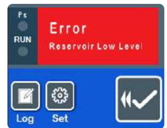
Error message of failures with full text display and access to log-book
