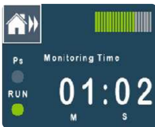
Lubrication time, shown in screen-saver mode. By swiping "Home" to the right, users can access the active mode
